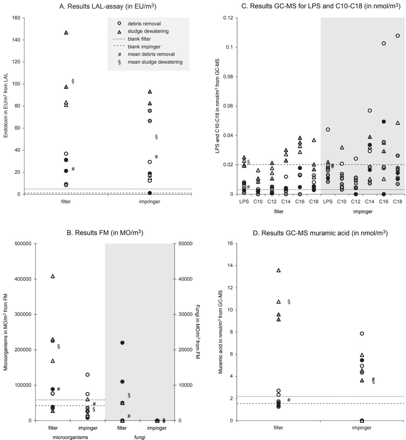
**Figure 2.** Comparison of results between 2 sampling methods (filters and impingers) per analytical method; the results are grouped by sampling location (● for debris removal and ▲ for sludge dewatering) and per sampling run (fill color).
