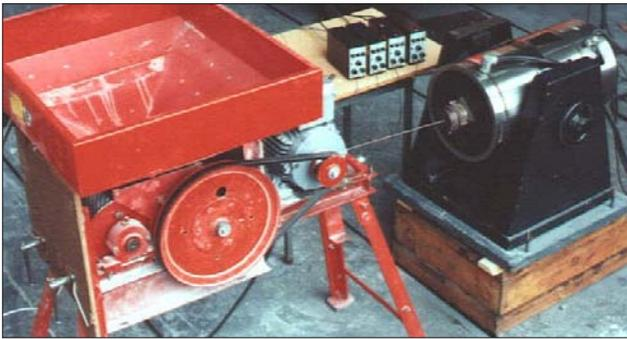
Figure 5. Forced vibration tests of grain crusher
