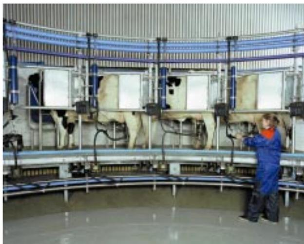
**Figure 2.** Milker's work position in the carousel. The platform (which can be raised and lowered to suit the height of the milker) is not shown. Copyright DeLaval Sales AB.
