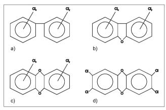
**Figure 1.** Structure of the individual groups POP representatives a) polychlorinatedbiphenyls (PCB), b) polychlorinateddibenzofurans (PCDF), c) polychlorinateddibenzodioxins (PCDD), d) 2,3,7,8- tetrachlorodibenzo-*p*-dioxin (TCDD). On the basis of [82]
