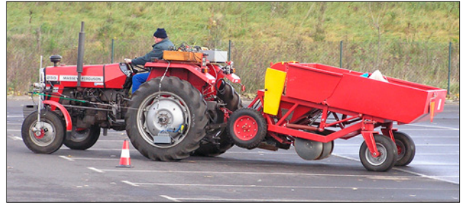
Figure 4. Semi-mounted potato planter during field work
