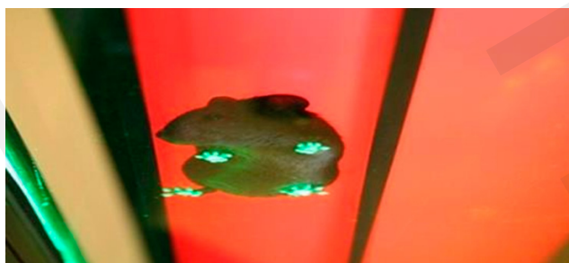
Figure 2. A mouse while walking on a Catwalk treadmill. The device during the test analyzes footprints on the treadmill, controlling the mechanism of locomotion. The green colors of the limbs are the result of diffraction of light emitted by diodes placed parallel to the glass surface of the treadmill, occurring at the point of contact between the limb and the glass surface.
