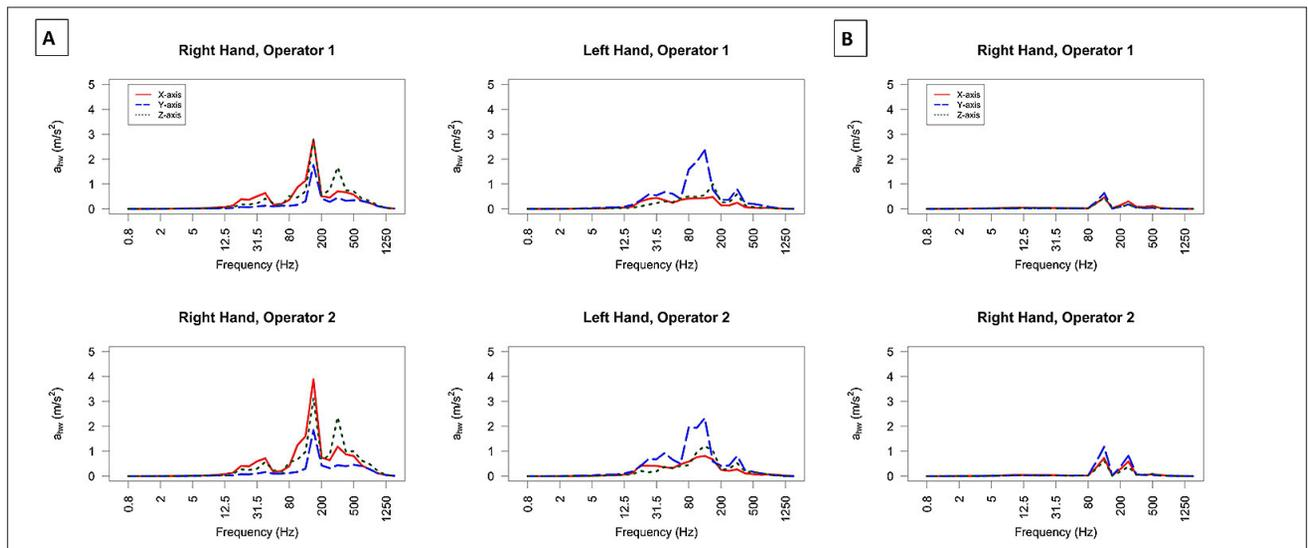
**Figure 4.**  $W_h$  weighted frequency spectra of bare hand: A – grass trimmer; B – backpack blower
