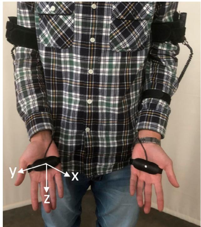
**Figure 2.** Operator wearing vibration dosimeters with 3 orthogonal axes shown
