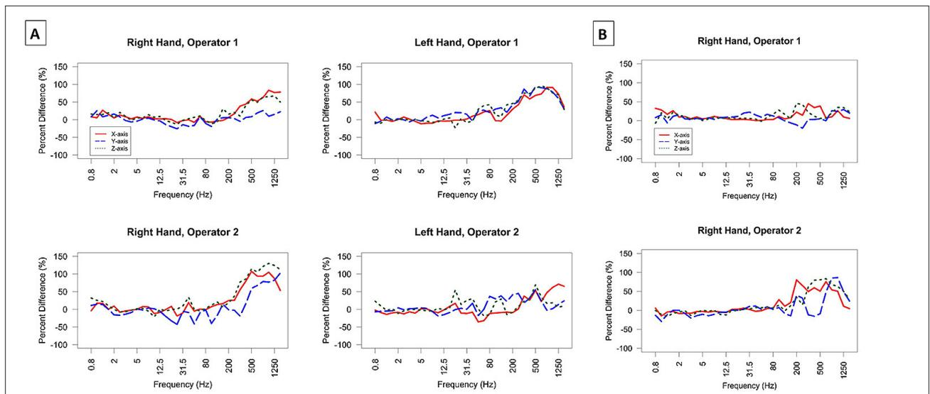
**Figure 5.**  $W_h$  weighted frequency spectra of acceleration percent difference (%): A – grass trimmer; B – backpack blower
