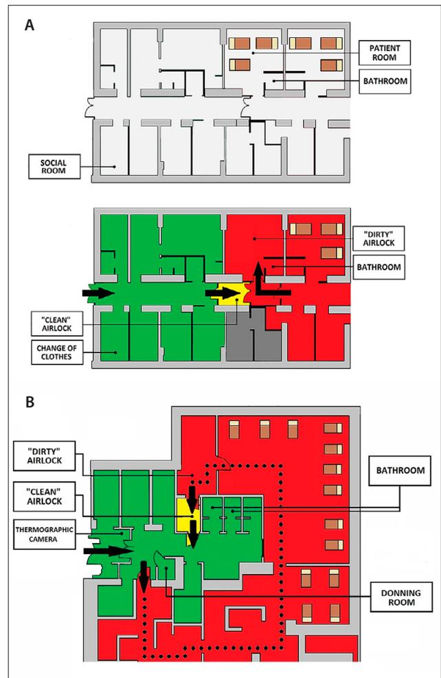
**Figure 6.** Work reorganization diagrams in two hospital exemplary units. A) Internal medicine department – view before (above) and after (below) reorganization. The airlock was created by placing walls across the corridor and excluding one of the patient rooms from use. B) Emergency Department – local conditions allowed the separation of entry and exit from the ward, introducing one-way traffic
