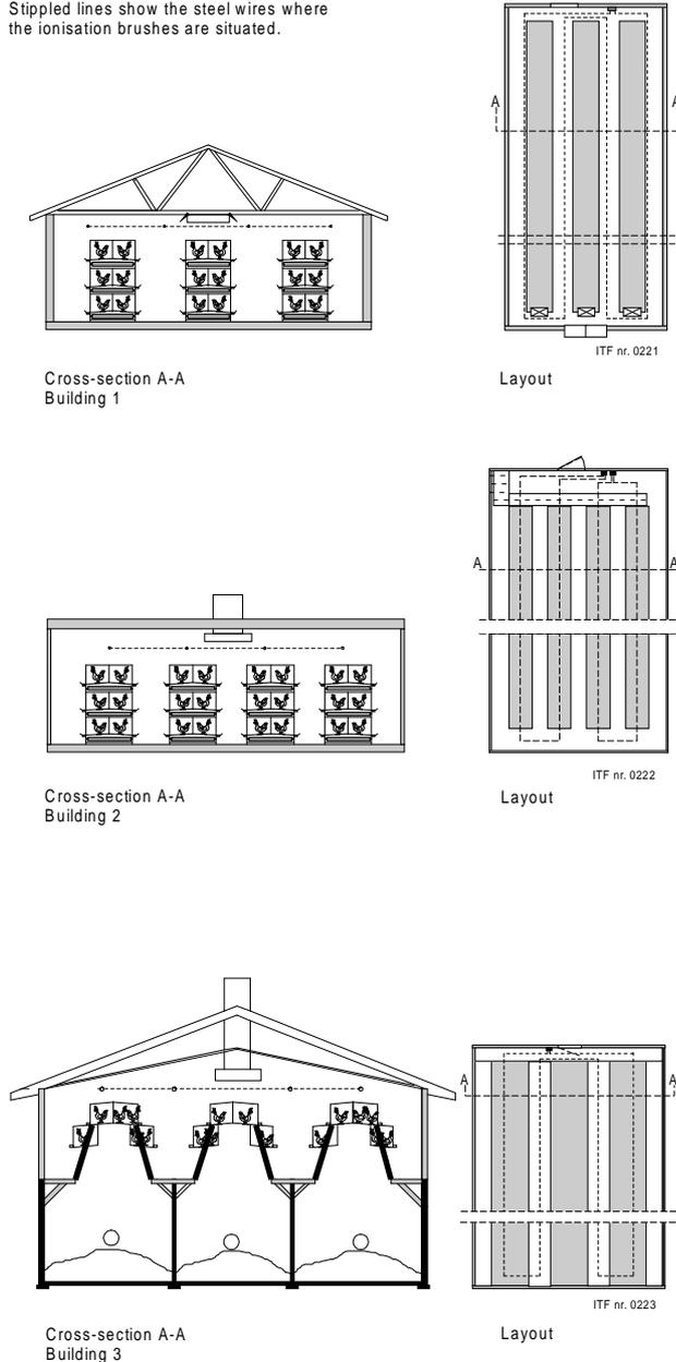
Figure 1. Cross-section and layout of the poultry confinement buildings.
