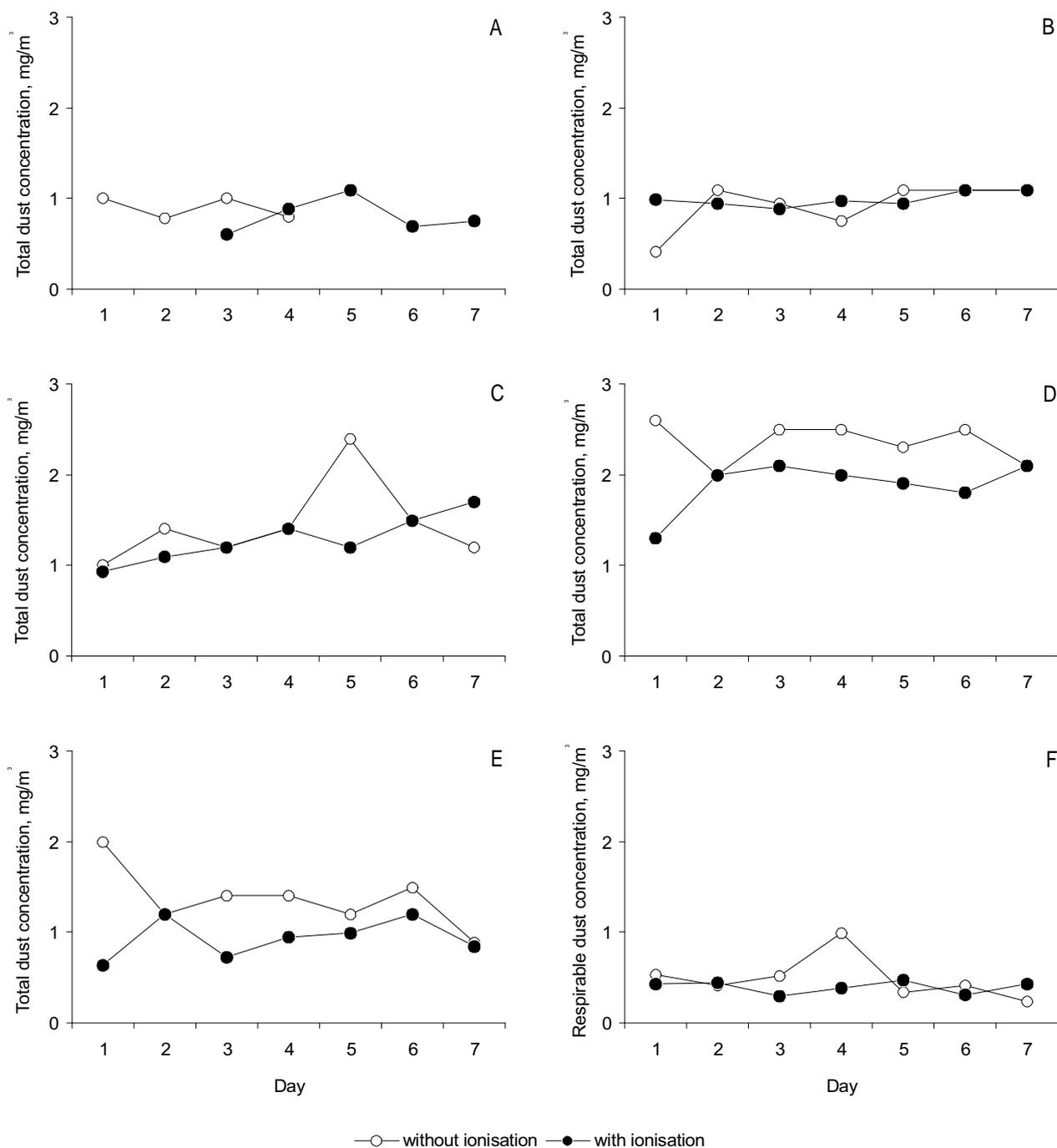
**Figure 2.** Dust concentrations measured during periods with and without ionisation. Total dust: (A) building 1, 1st experiment, (B) building 1, 2nd experiment, (C) building 2, 1st experiment, (D) building 2, 2nd experiment, (E) building 3. Respirable dust: (F) building 2, 2nd experiment.
