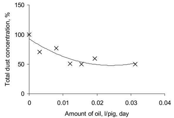
**Figure 11.** Relative changes in dust concentration when an automatic oil spraying system has been used.
