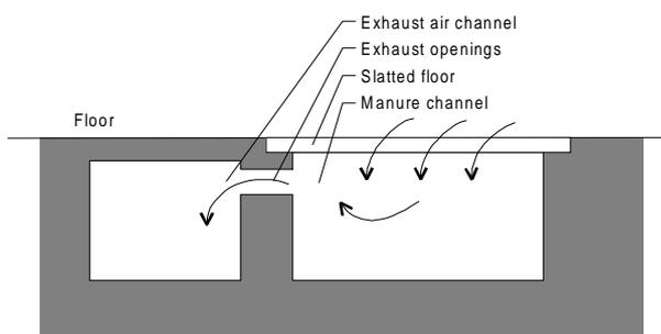
**Figure 4.** Two investigated principles for manure gas exhaustion.
