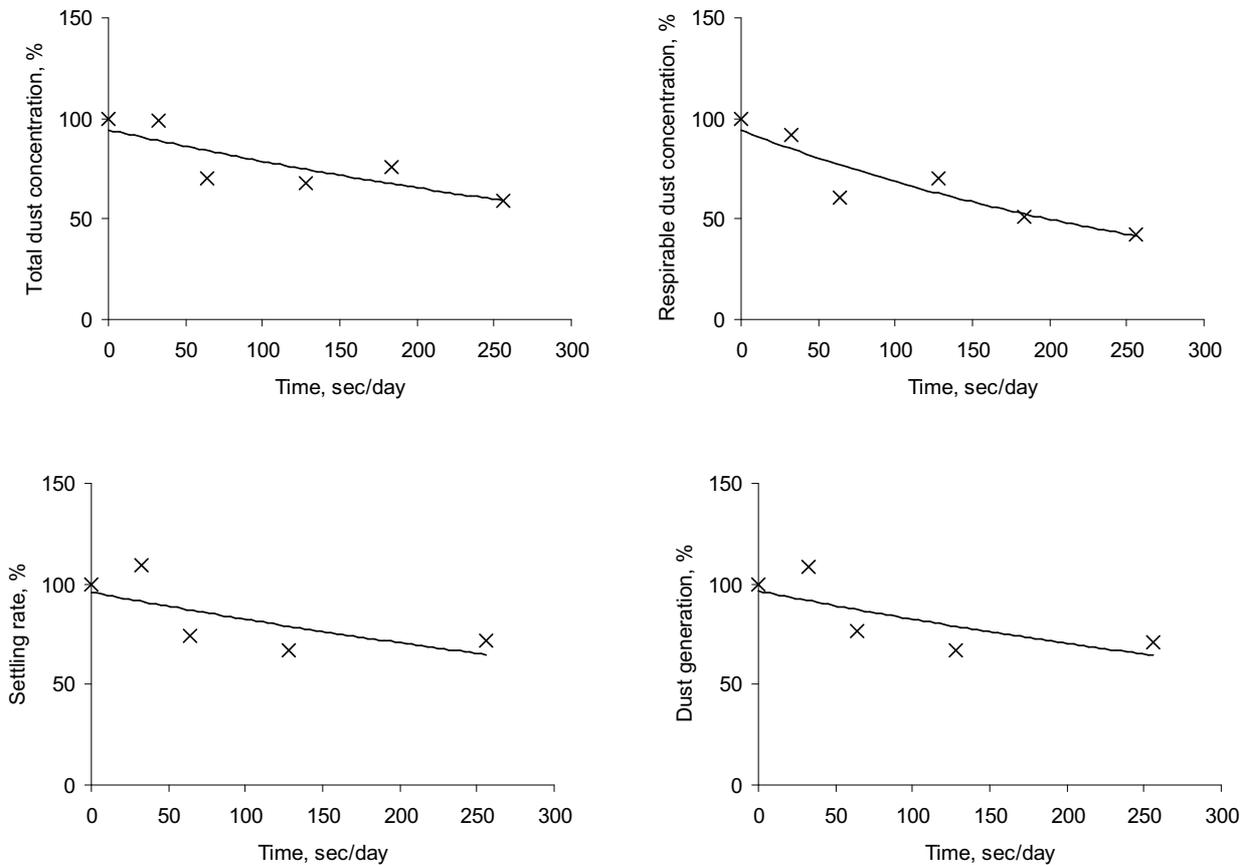
**Figure 10.** Influence of humidification on total and respirable dust concentrations, settling rate and generation of dust as a function of the spraying period when full cone nozzles were used (reference level is 100%).
