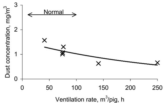
**Figure 8.** The influence of ventilation rate on total dust concentration in a building for growing-finishing pigs with an average body weight of  $67.0 \text{ kg}$ .
