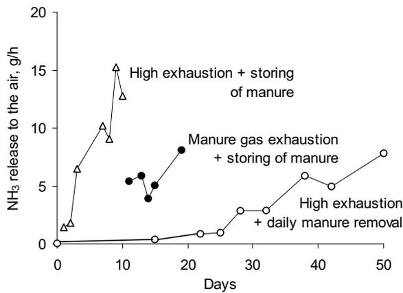
**Figure 14.** The influence of manure storage time on conveyors on ammonia release in an aviary system for laying hens when ventilation air is exhausted at roof level (high exhaustion) and when the air is exhausted through an air duct close to manure conveyors (manure gas exhaustion).
