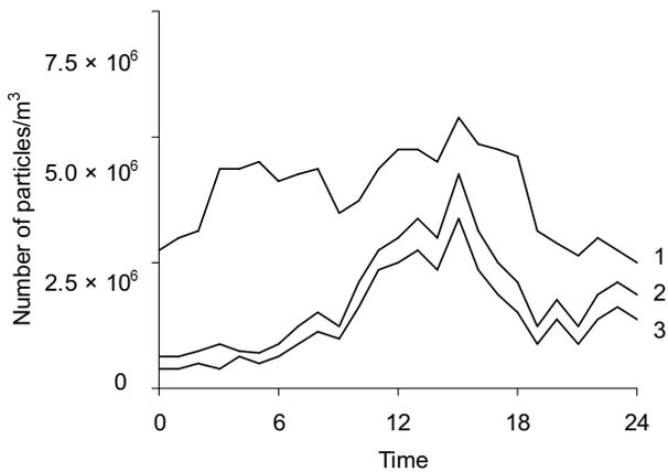
**Figure 5.** Daily variation in the number of dust particles at constant ventilation rate ( $75 \text{ m}^3/\text{pig, h}$ ) in a building for growing - finishing pigs. Line 1 – Particle size  $0.5\text{--}1.0 \text{ }\mu\text{m}$ ; Line 2 – Particle size  $1.0\text{--}2.0 \text{ }\mu\text{m}$ ; Line 3 – Particle size  $2.0\text{--}5.0 \text{ }\mu\text{m}$ .
