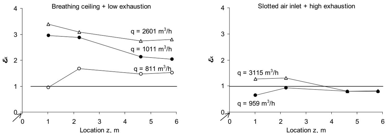
**Figure 15.** Ventilation effectiveness ( $\epsilon_x$ ) at different distances from the injection point of an air pollutant ( $z$ , m) at two combinations of air inlets and air outlets. The pollutant is released at the arrow.  $q$  = ventilation rate,  $m^3/h$ .
