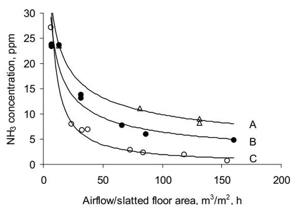
**Figure 13.** Ammonia concentrations according to airflow rate when the air is exhausted with a fan in the wall (A), exhausted through a separate exhaust air duct (B), and exhausted through the manure channel (C) in a house for growing-finishing pigs.
