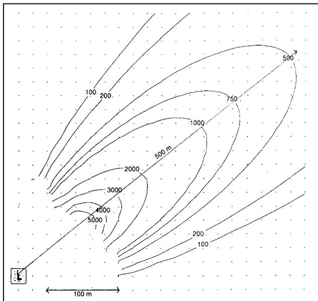
**Figure 2.** Prediction of microbial immissions in the vicinity of a compost plant (airborne bacteria) according to TA-Luft. L = source of emission. Curves with numbers = calculated concentrations of airborne bacteria (cfu/m<sup>3</sup>).
