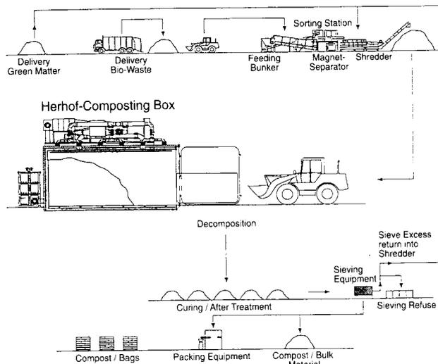
Figure 1. Display of biowaste decomposition with the Herhof box system.
