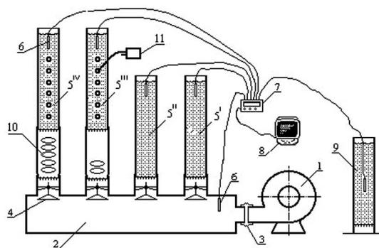
**Figure 1.** Schematic diagram of drying test rig: 1 – air blower; 2 – chamber with constant static pressure; 3 – flexible joint; 4 – restrictor; 5<sup>I</sup>, 5<sup>II</sup>, 5<sup>III</sup>, 5<sup>IV</sup> – ventilated cylinders with grain; 6 – temperature sensors and moisture content; 7 – secondary ALMEMO measurement unit; 8 – computer; 9 – natural ventilation cylinder with grain; 10 – ozonators; 11 – measurement unit of ozone concentration.
