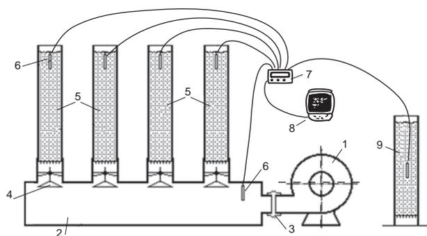
**Figure 1.** Principal scheme of shaft drier: 1 – ventilator; 2 – constant static pressure chamber; 3 – flexible joint; 4 – valve; 5 – ventilated cylinders filled with grain; 6 – temperature and humidity sensors; 7 – secondary ALMEMO meter; 8 – computer; 9 – natural ventilation cylinder filled with grain.
