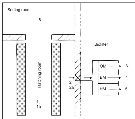
**Figure 2.** Place of collected air samples. 1-6 – sampling points. OM – organic medium, BM – medium with bentonite, 5 – medium with halloysite.
