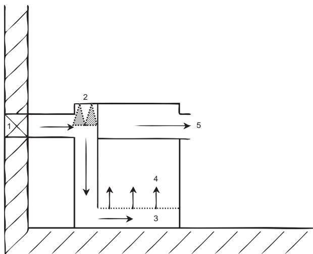
**Figure 1.** Schematic diagram of biofilter. 1 – fan, 2 – humidifier, 3 – air distribution, 4 – biofilter media, 5 – outlet gas.
