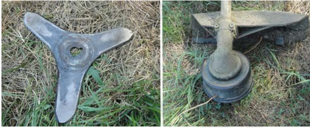
Figure 1. The employed cutting heads used during trials: brush knife (left) and mowing head (right)
