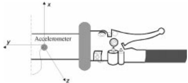
Figure 2. Accelerometer position during vibration measurement with marked directions.
