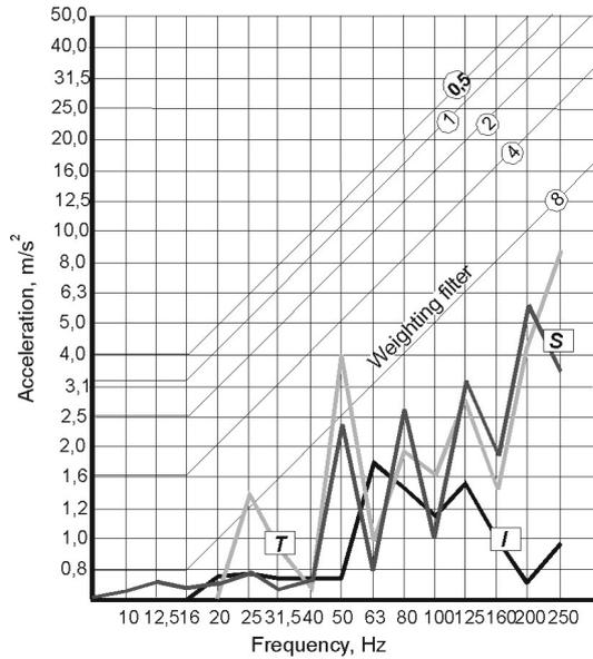
**Figure 6.** Graphic representation of vibration levels in z-direction (I - idling, T - transportation, S - soil tillage).
