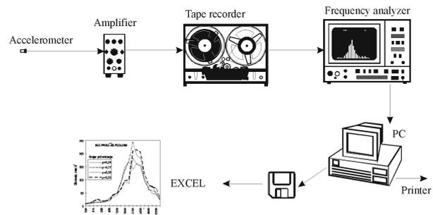
Figure 3. Schematic presentation of the equipment used for vibration measurements and analysis.
