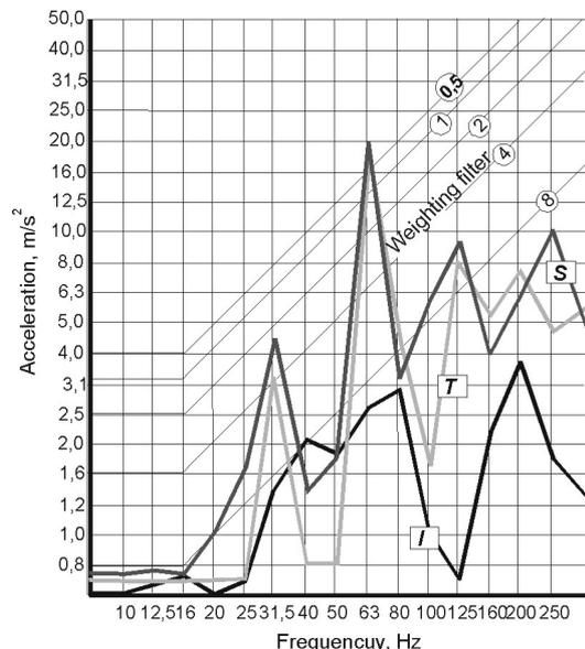
**Figure 5.** Graphic representation of vibration levels in y-direction (I - idling, T - transportation, S - soil tillage).
