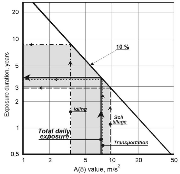
**Figure 7.** Vibration exposure for predicted % prevalence of vibration-induced white finger in a group of exposed persons (I - idling, T - transportation, S - soil tillage).
