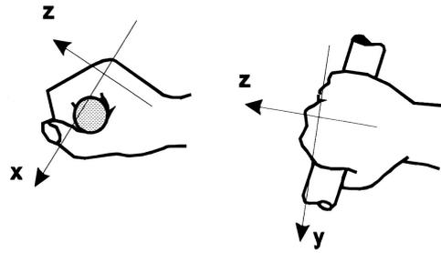
Figure 1. Orientation of the axes for the vibrations measurement (according to ISO 5349).
