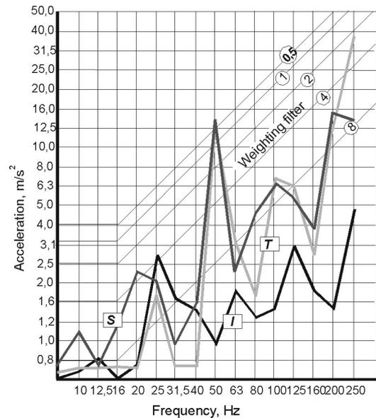
**Figure 4.** Graphic representation of vibration levels in x-direction (I - idling, T - transportation, S - soil tillage).
