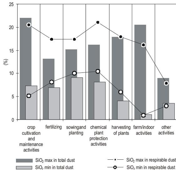
Figure 3. Percentage of SiO<sub>2</sub> in airborne dust.
