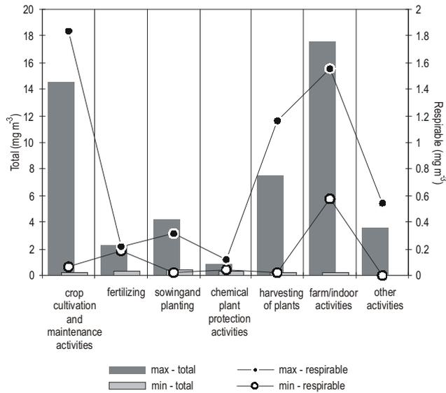
Figure 4. Concentration of free silica  $\text{SiO}_2$  in respirable zone.
