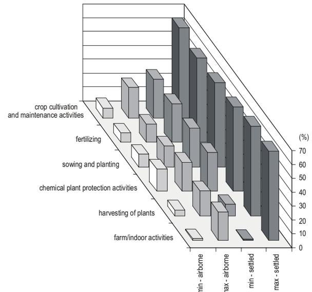
Figure 5. Level of  $\text{SiO}_2$  in settled and airborne dust in respiratory zone.
