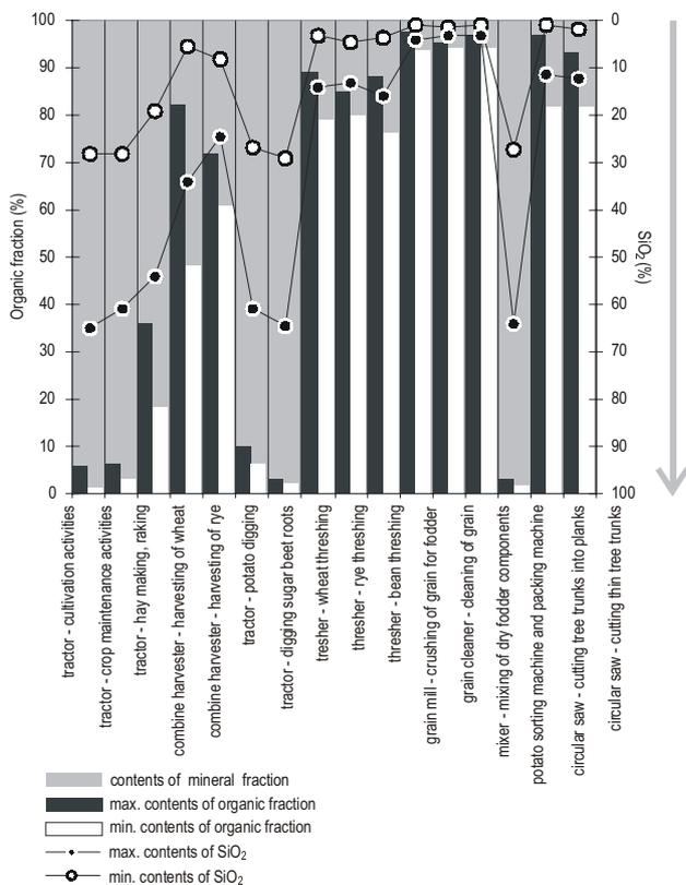
Figure 2. Contents of organic and mineral fractions, and free silica SiO<sub>2</sub> in settled dust.
