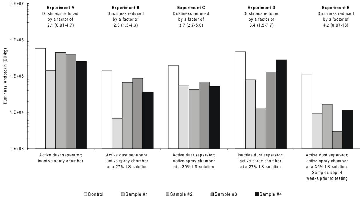
**Figure 6.** Dustiness of chopped straw (barley) in terms of endotoxin units (EU) emitted per unit mass (kg) of straw. Dustiness is given versus techniques to reduce the dustiness. The factor of reduction in dustiness is given with reference to the control sample, presented as the geometric mean; 95% confidence interval in parentheses.
