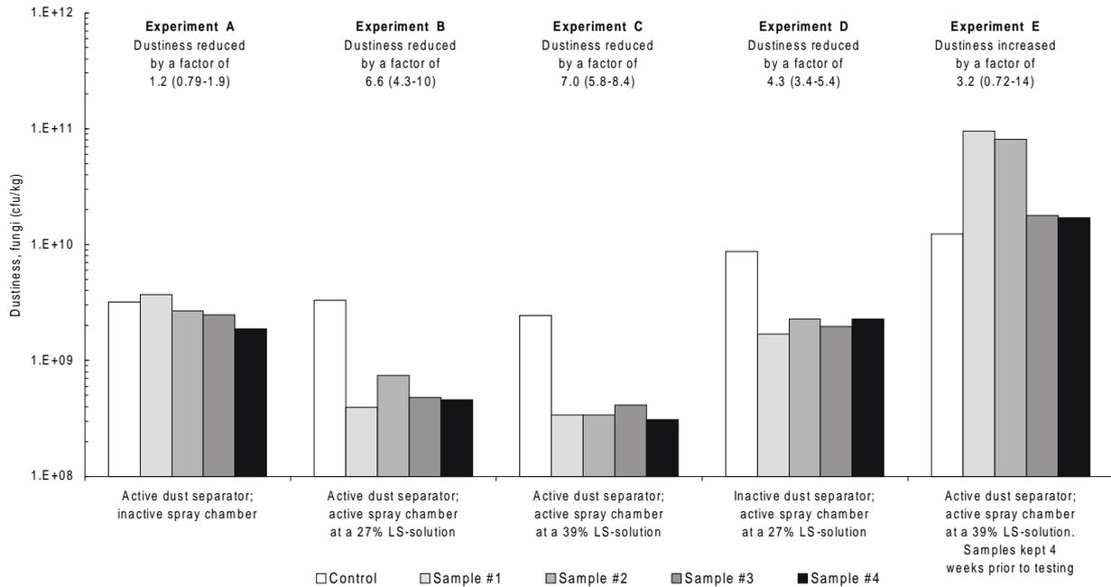
**Figure 5.** Dustiness of chopped straw (barley) in terms of colony forming units (cfu) of fungi emitted per unit mass (kg) of straw. Dustiness is given versus techniques to reduce the dustiness. The factor of reduction in dustiness is given with reference to the control sample and is presented as the geometric mean; 95% confidence interval in parentheses.
