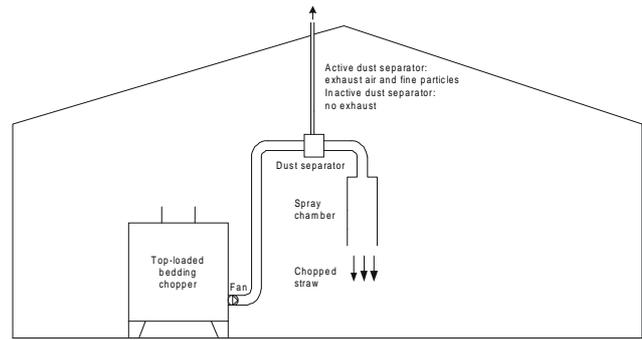
**Figure 1.** Experimental set-up (not to scale). The bedding chopper was fitted with a dust separator and a spray chamber.
