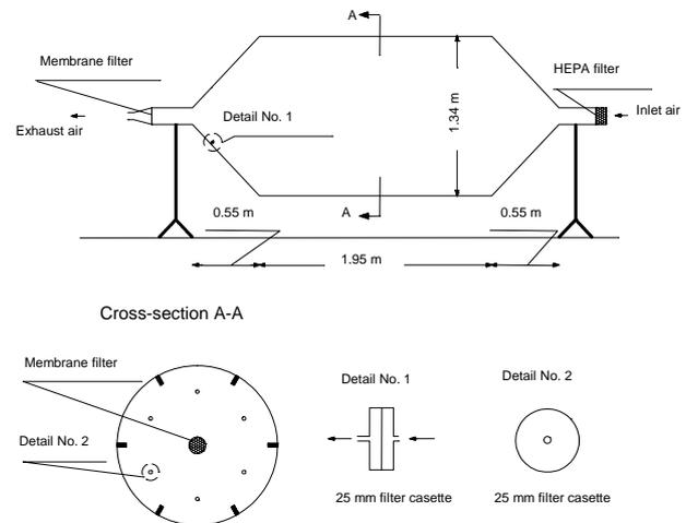
**Figure 2.** Rotating drum dustiness tester. The drum was operated at 7 rpm at an airflow rate of 420 l min<sup>-1</sup>.
