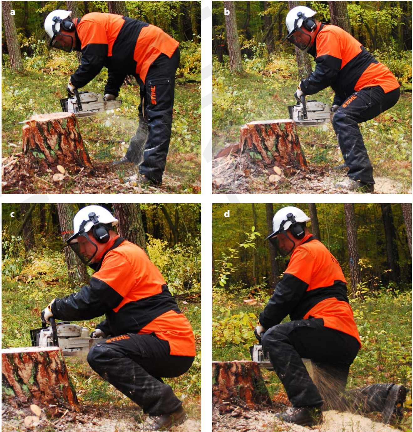
Figure 1. Body postures selected for the measurement of physiological load during tree cutting: a – back bent forward with straight legs (stoop), b – back bent forward with bent legs (flexed-stoop), c – squat, d – kneel on one knee (half-kneel). Photo by W. Grzywiński
