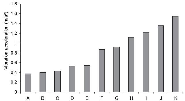
**Figure 2.** Equivalent values of vibration acceleration for different work activities. (A – cutting and grinding of maize; B – combine harvesting of cereal crops; C – beetroot digging; D – working with tractor front loader; E – potato digging; F – spreading of fertilizers; G – grass mowing; H – disc harrowing; I – transportation of manure (field road); J – hay tedding and raking; K – transport 2 trailers (asphalt road).)
