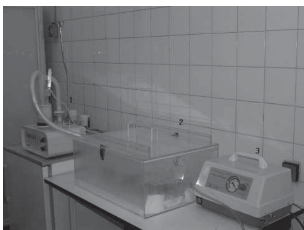
Figure 3. An inhalation challenge set for mice during inhalation. The chamber is filled with nebulized allergen extract.
